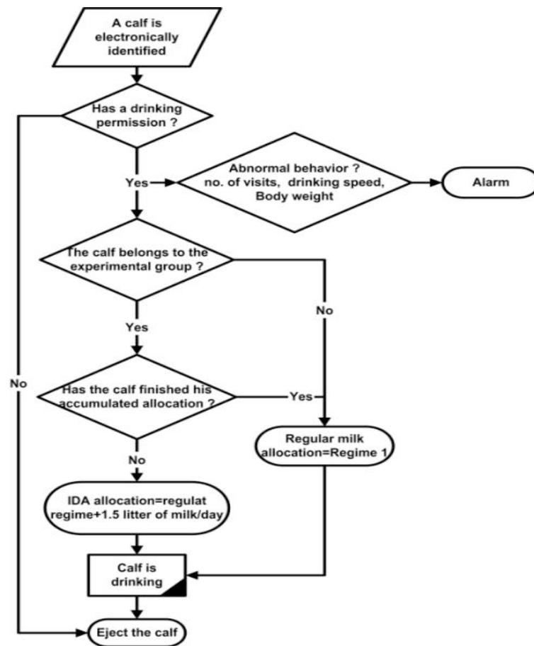
**Fig. (3).** Materials and methods. Control system, software implementation flowchart - from the moment a calf has identified at the drinking machine entrance till he received milk or ejected from the machine
